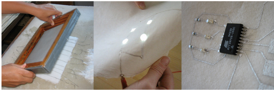
Fig. 1. Left: paper and conductive threads composite; center: flexible paper display; right: paper-based printed circuit board (PPCB).
